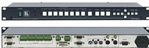
The **VP-724xl** is an 8-input scaler/switcher with unbalanced stereo audio. It scales any composite, s-Video (Y/C), component video (YUV), DVI video or computer graphics video signal up or down to a selectable graphics or HDTV output resolution and provides glitch-free switching between sources through FTB™ (fade-thru-black) switching technology.
